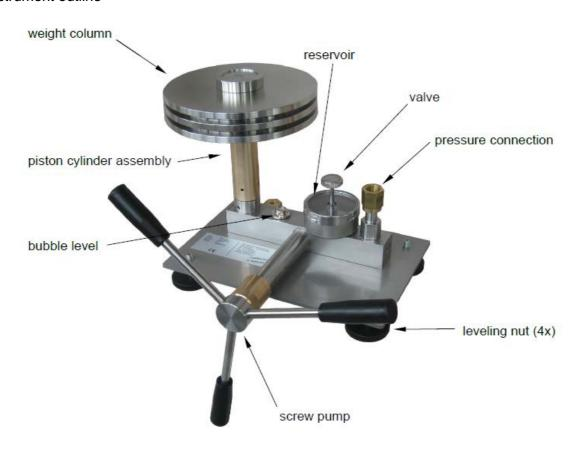
To change from low pressure range to the high pressure range it is necessary to change the piston cylinder assembly.
