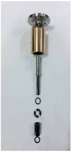
Piston assembly with large diameter = 10 mm
