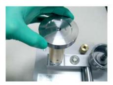
4. Unscrew the piston cylinder assembly with the hook wrench.
